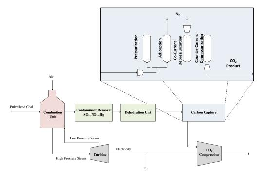
In order to examine the effectiveness of hydrophobic materials for carbon capture, we will investigate several different hydrophobic adsorbent (e.g. activated carbon, ZIF-8) and calculate the cost of capturing CO2 under dry and humid conditions with a Fractionated Vacuum Pressure
