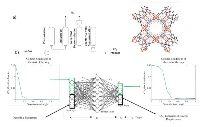
**Figure 1.** (a) Diagram of one potential PSA cycle and the metal organic framework (MOF) material; (b) schematic of the ANN surrogate model. For each step, the ANN surrogate model will take the initial conditions of the column along with operating parameters for that step (e.g. length of column, operating pressure, time length) and will estimate the conditions of the column after the step along with the gas emitted/consumed during the step and the energy requirements.
