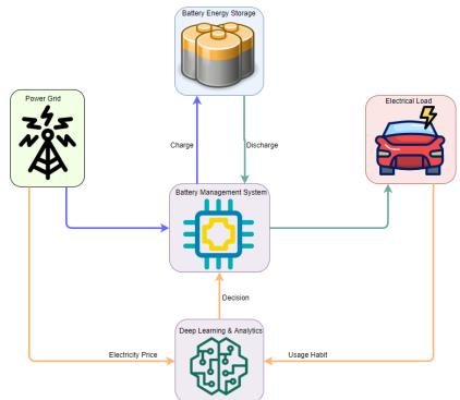
In this project, we aim to leverage the power of deep learning and system analytics to extract some useful information from the past data and integrate with the battery model to extend the lifespan of the battery energy storage system while fulfilling the power demand and maximizing the economic benefit. The case study will be based on the electric vehicle which comprises the vehicle model and the battery model.
