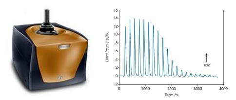
Nano ITC table-top instrument (TA Instruments) and calorimetric spectrum in case of exothermal complexation.
